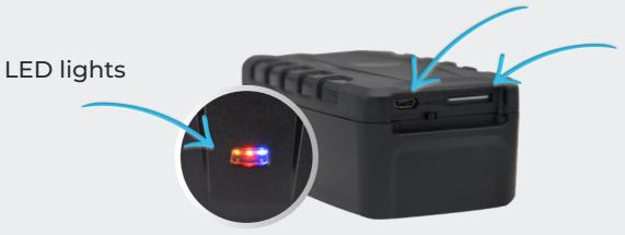
Before using it for the first time, you should charge the GPS tracker for about 8-12 hours. Connect the supplied charging cable to the charging port on the GPS tracker. Then attach the USB port to the power socket adapter. Once the GPS tracker is connected to the power source, please charge it until the red LED turns off.
